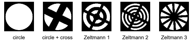
Figure 1: Simulated condenser apertures. From left to right: Standard circular aperture, standard aperture with a cross in the center, bullseye aperture (4 rings), bullseye aperture (8 rings), ray aperture. The last three apertures are inspired by Zeltmann et al. [8].
